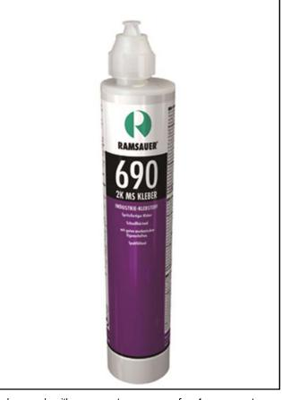
can be used with any customary gun for 1-component compounds. 690 2-K-MS KLEBER does not contain any solvents, isocyanate or silicone. The adhesive cures virtually without any odour and can be ground and covered with paint coats once it has cured completely.
